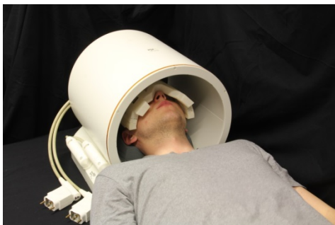
Figure 1: Whole setup which was used to obtain high-resolution ^{23}\text{Na} images of the human eye at 7.0 Tesla along with proton anatomical reference images: the 6-channel transceiver array ( ^{23}\text{Na} ) placed on the volunteer's head inside the volume coil ( ^1\text{H} ).
