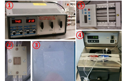
Fig.1: 1) Gas mixing station, 2) bioreactor housing, 3) polymer chip (DYNARRAYS(R)), 4) water bath and 5) perfusion pump are shown 3 .
