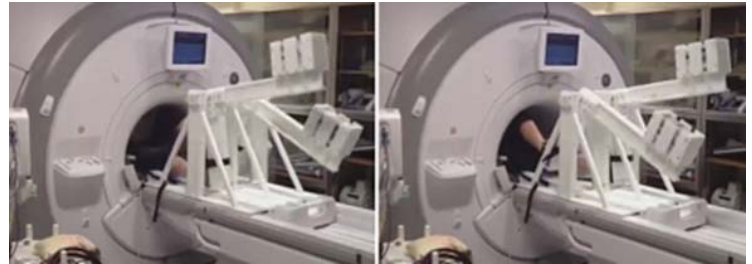
Figure 1: MRI-compatible exercise equipment. The subject follows a dynamic stepping motion to the beat of a metronome. Workload is determined by the cadence, step length, and the amount of removable weights added to the end of each lever arm.
