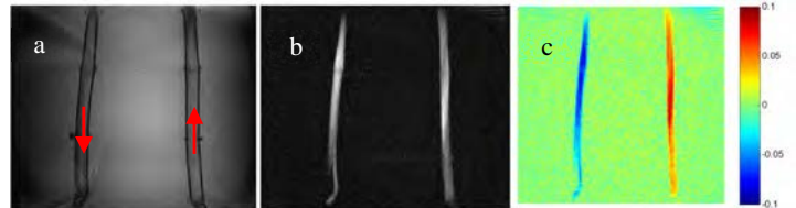
Figure 2. Flow phantom images: (a) reference image acquired using FA 0^\circ BIR-4; (b) magnitude image acquired with VSP; (c) phase sensitive image depicting flow direction.
