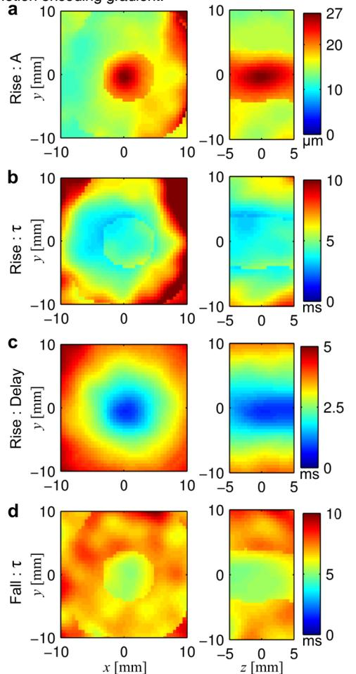
**Figure 2:** Orthogonal slices through 3D parameter maps derived from dynamic 3D ARFI tissue response measurement. (a) Steady-state tissue displacement, (b) Time constant of exponential displacement during rise, (c) Delay-offset before displacement begins relative to start of pulse, (d) Time constant of exponential tissue relaxation.
