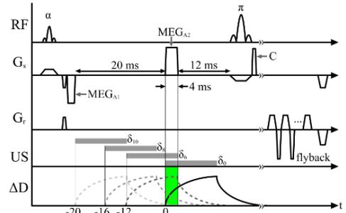
**Figure 1:** Dynamic 3D SE ARFI pulse sequence. Multiple snapshots of tissue displacement were acquired with varying delays between the US and motion encoding gradient.
