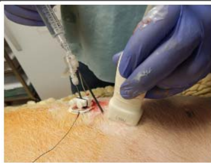
Figure 1: A paracentesis catheter is inserted into a pig kidney under ultrasound visualization for placement of a fiber-optic O_2 probe. Customized plastic clamps secured the probes to limit their movement after placement.
