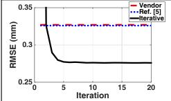
Fig. 2) Fiducial marker root-mean-square-error (RMSE) versus iteration number. Note the rapid, monotonic convergence of the GN algorithm.
