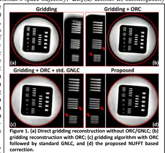
Figure 1. (a) Direct gridding reconstruction without ORC/GNLC; (b) gridding reconstruction with ORC; (c) gridding algorithm with ORC followed by standard GNLC, and (d) the proposed NUFFT based correction.
