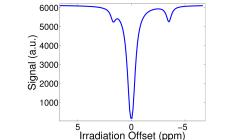
**Figure 1:** Simulation results showing the application of matrix-algebra-based model using a 3 spin-pool approach (with NOE between water and spin pool at -3.5ppm, and CEST between water and spin pool at 1.7ppm).
