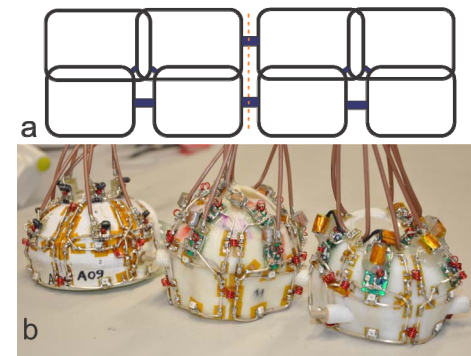
Fig.2: a) 2D view of the receive coil layout. The thick bands represent inductive decoupling. The helmet could be split along the dotted line in two halves because there is no geometric overlap between the two halves of the coil. b) 8-channel receive arrays adapted to specific animal head shapes.
