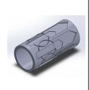
Fig 1. SolidWorks rendering of former with etched pattern of coils and tune/match boards
