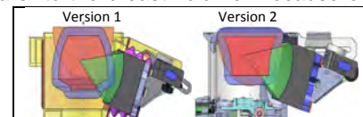
Figure 2. Treatment volumes for v1 (left) and v2 (right). Pink volume is treatment volume achieved with mechanical steering, purple volume is additional volume achieved with electronic steering.
