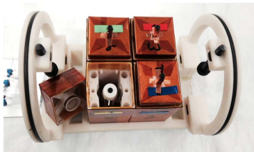
Fig. 2: Four shielded coil system, with one open shield.
