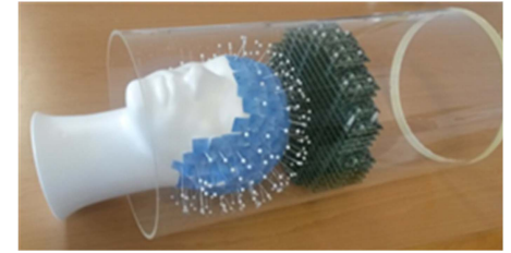
Figure 1: Concept of the 256 channel receiver coil. The blue squares indicate the size and position of the coil elements. The pre-amplifier boards (green) are stacked behind the head and are small enough to fit inside the transmit coil.
