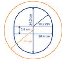
Figure 1: dimensions of 8 channel receive-only loop array (dark blue) and outer dipole array (orange)
