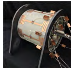
Figure 3: structure of combined dipole and loop array
