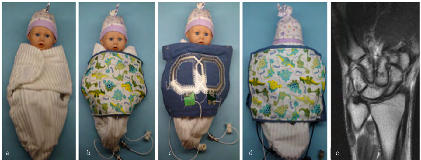
Figure 1. Left to right: a) Newborn-sized doll in a swaddle. b) Pouch, with Veltex backing, attached to the front of the swaddle. c) Inside view of the pouch. d) Second pouch and coil pair attached to the doll's back for a 4-channel array. e) Adult human wrist imaged with the coil pair shown in c).
