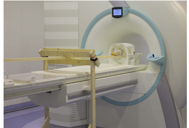
Fig. 1: Wooden frame used for decoupling. The phantom was fixed on the bar, so that the effect of scanner vibrations was minimized.
