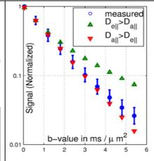
Fig 2: Decay curves for isotropic encoding scheme. The blue dots with error bars are log averaged data for all WM voxels measured with the isotropic encoding sequence. The upper and lower triangles are the estimated curves from the two fitting conditions.
