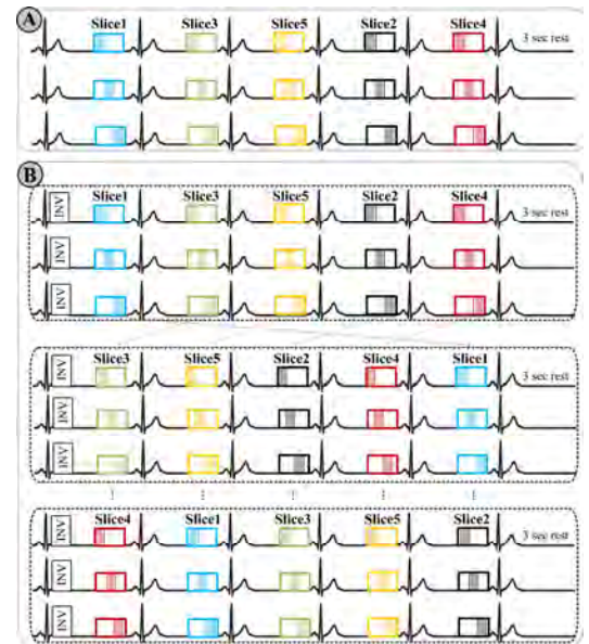
Figure 1. Sequence scheme of the proposed multi-shot STONE sequence. (a) Each slice is first acquired without any magnetization preparation pulse (b) Each IR block consisted of non-selective inversion pulse and slice-selective excitation is repeated for all segments and the order of slices is shifted cyclically through.
