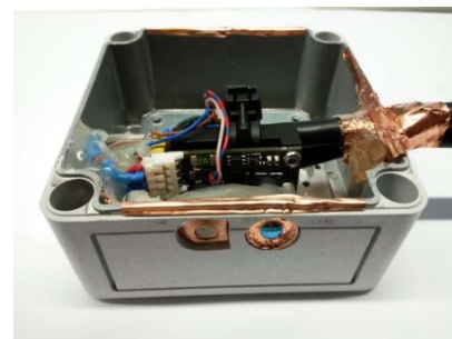
Fig. 1: Modified and shielded ToF camera.
