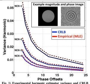
Fig. 1) Experimental harmonic estimator variance and CRLB predictions for various phase offset and NEX combinations.
