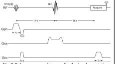
Fig.2 Pulse sequence diagram for the implementation of Chirp modulated Fourier encoding.
