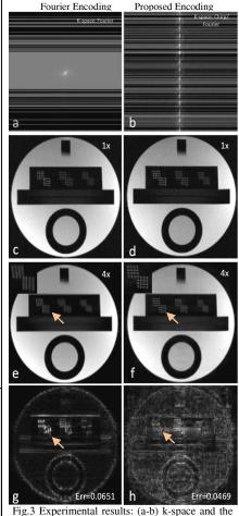
under-sampling pattern, c-d fully sampled images, (e-f) CS reconstructed images with 4x acceleration factor, (g,h) relative error.
