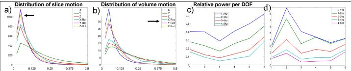
Fig 1: distribution of individual head motions (mm, deg) for a) slicewise and b) volumetric motion for 6 DOF, c) shows relative power per DOF (1=X, 2=Y, etc) in each frequency band (each band is normalized to 0-1Hz band), d) shows non-normalized power
