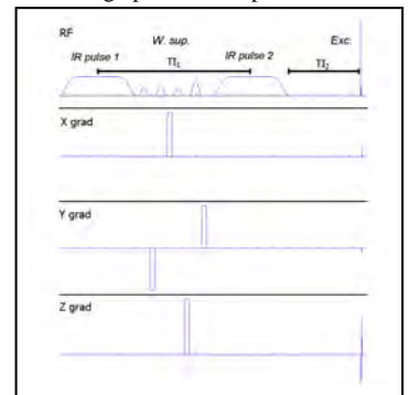
Fig.1: Pulse sequence design composed of DIR, WS, and FID excitation
