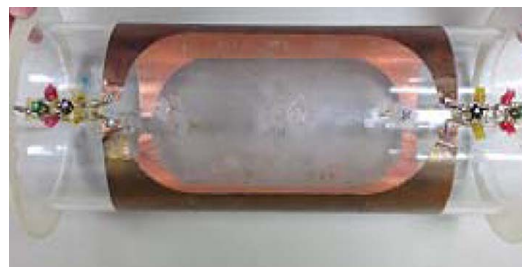
Figure 1. The parallel-plate waveguide for multinuclear spectroscopy.
