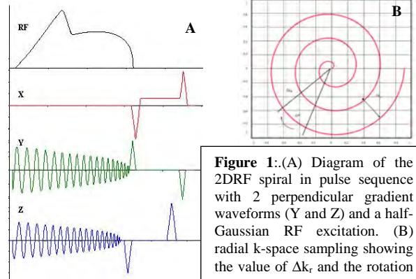
**Figure 1:** (A) Diagram of the 2D RF spiral in pulse sequence with 2 perpendicular gradient waveforms (Y and Z) and a half-Gaussian RF excitation. (B) radial k-space sampling showing the value of  $\Delta k_r$  and the rotation angular variable  $\theta$ .
