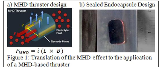
Figure 1: Translation of the MHD effect to the application of a MHD-based thruster
