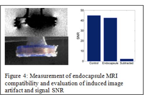
Figure 4: Measurement of endocapsule MRI compatibility and evaluation of induced image artifact and signal SNR
