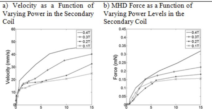
Figure 3: Quantification of system dynamic performance using the preliminary raft design. Power is scaled to required 3T levels based on data acquired at lower field strengths: (a) peak velocities under varying power levels, (b) and MHD force.
