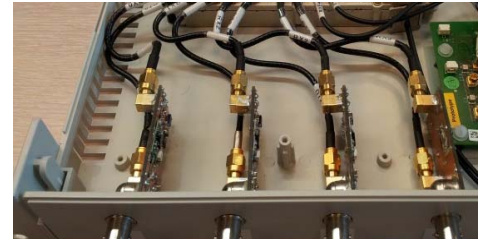
Figure 1. Photograph of external preamplifiers with SAW filters at 298MHz (7T) connected to the adapted digital 1.5T receivers.
