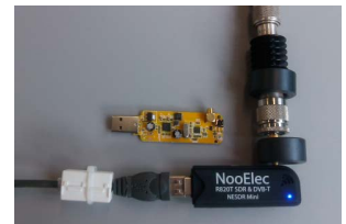
Fig. 1: DVB-T stick with ferrite cores, and input attenuator.
