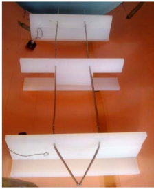
Fig. 2: Experimental setup. Cable shields of the both pick-up loops are grounded at the copper tube.
