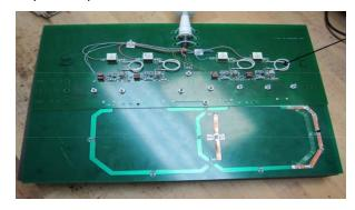
We built and tested a sliding coupler system for connecting one or two magnetically decoupled octagonal 4" coils to two QED preamps, which fed two receive channels of a 1.5T Siemens Magnetom Espree MRI scanner. The vendor supplied standard image reconstruction software was used.
