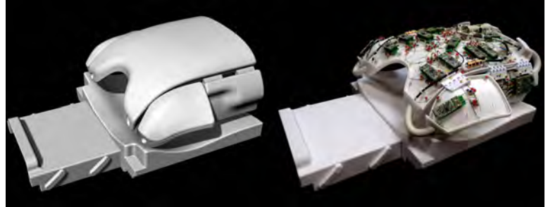
Fig.1: 3D coil model and constructed 64-channel cardiac coil array
