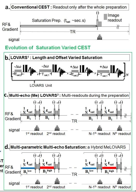
**Fig.1** Comparison of conventional (a) and the evolution of our saturation-varied CEST schemes, from LOVARS (b), MeLOVARS (c) to the proposed Multi-parametric Multi-echo saturation (MMS) (d), for fast image acquisition of images with interleaved  $B_1$  to modulate CEST contrast.
