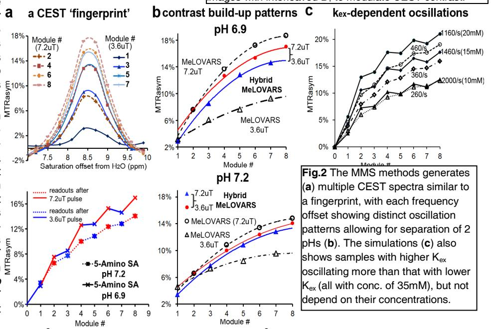
**Fig.2** The MMS methods generates (a) multiple CEST spectra similar to a fingerprint, with each frequency offset showing distinct oscillation patterns allowing for separation of 2 pHs (b). The simulations (c) also shows samples with higher  $K_{\text{ex}}$  oscillating more than that with lower  $K_{\text{ex}}$  (all with conc. of 35mM), but not depend on their concentrations.
