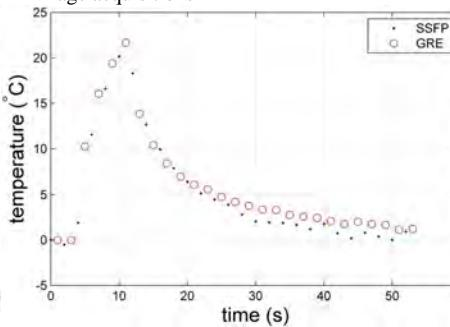
**Fig. 3:** Temperature evolution during 1s sonifications measured by fast bSSFP and GRE sequences.
