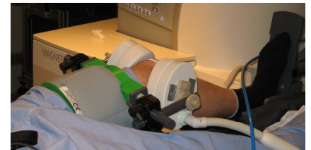
Fig. 1: Setup for the MRI experiments with in situ mechanical knee loading.
