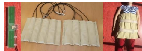
Figure 1: 8 channel TxRx radiative Antennas used in this study. From left to right: Single antenna, all 8 channels and the positioning on the patient.
