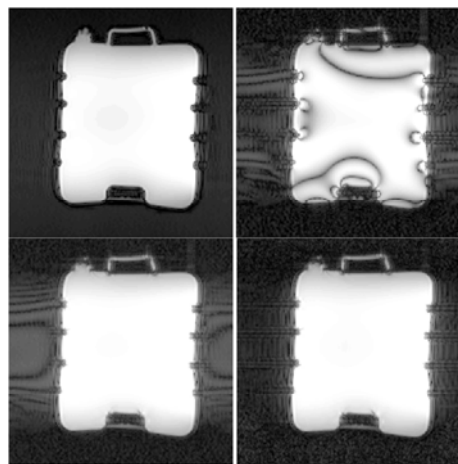
Fig. 2 Images obtained in phantom with the ASE-prepared HASTE. Top: in-phase images ( S_{\parallel} ) acquired with \tau=0 ms (left) and \tau=10 ms (right). Bottom: combined images S(\tau)=\sqrt{S_{\parallel}^2 + S_{\perp}^2}/2 acquired with \tau=10 ms, before ghost elimination (left) and after ghost elimination (right).
