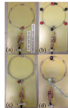
Fig. 1 Proposed RF-shim loop geometries (a) conventional loop, (b) RF-shim loop with chokes, (c) coaxial loop, (d) concentric loop.
