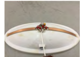
Figure 5: Constructed 3D curved dipole prototype with substrate filled with distilled water
