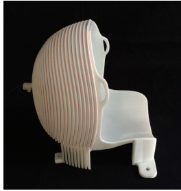
Figure 1: 3D printed single channel volume head coil. The coil was used for both transmit and receive at 276 kHz (6.5 mT)
