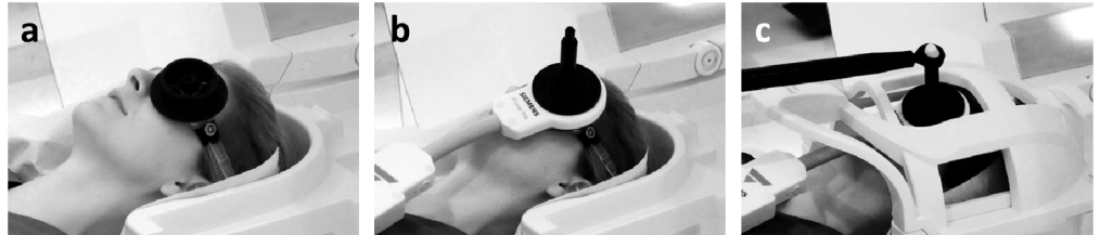
Fig. 1: Driver setup for MRE of the eye. The modified goggle fits inside the head coil and is connected with a carbon fibre rod to a piezo ceramic based driver [4] placed at the foot end of the patient table.
