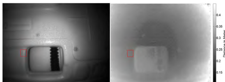
Figure 1: Intensity (left) and depth (right) image of the camera; The ROI used for respiratory motion tracking is indicated by a red box.
