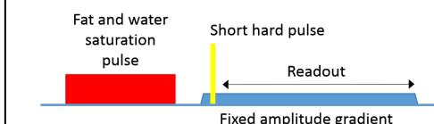
**Figure 1.** Schematic plot of the WASPI sequence. (1 TR)
