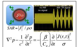
Fig.1 Rapid RF heating causes thermal expansion. If MRI RF is AM modulated at 1 MHz, a continuous 1 MHz thermo-acoustic (TA) pressure wave is created. Cp~4e3 J/kgK, β=4e-4K<sup>-1</sup>, c~1500m/s,
