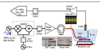
Fig 3: Setup to amplitude modulate (AM) 64 MHz carrier at 1 MHz center with 375 kHz span. Tip lead is toroid driven in saline, or strip-line coil excites below saline phantom.
