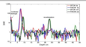
Fig 4:) FMCW (250x4ms, 375 kHz chirps) and SFCW (250 tone x 2ms x 2 Nex,) of strip-line SAR, and RF tip-heating TA signal.
