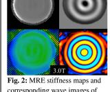
**Fig. 2:** MRE stiffness maps and corresponding wave images of water based gelatin phantom obtained at 1.5T (top) and 3.0T (bottom) using 2D-GRE sequence. Stiffness values (kPa) were 3.4 at 1.5T and 3.2 at 3.0T.
