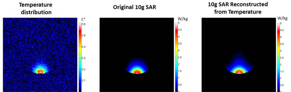
**Figure 1:** Spatial distributions of temperature increase affected by noise (left), 10g SAR average which generated the temperature distribution (center), reconstructed 10g SAR from the noisy temperature distribution (right).
