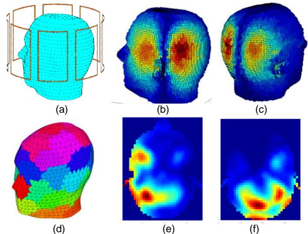
Figure 2. (a) The eight-channel loop array model with the "Duke" head. (d) The decomposed sub-domains in fast MoM simulation. (b,d) The induced equivalent currents on the head surface. (e,f) The associated peak local SAR in the head.
