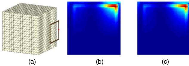
Figure 1. Layered cubic phantom model and a loop coil (a), local SAR maps computed by the conventional FDTD (b) and our proposed method (c).
