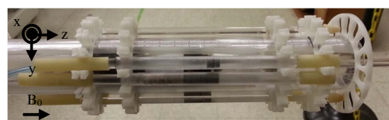
Figure 2. The shim frame used to implement passive shim configurations. Shim elements are positioned using hollow plastic rods mounted onto the frame.
