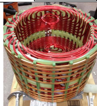
Figure 2. Completed windings of gradient coil.
