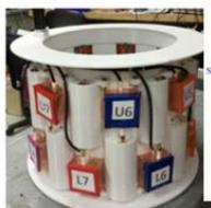
Fig 1: 16-channel Tx array prototype
